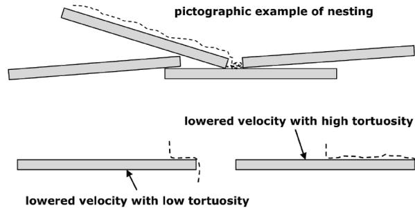
Fig 8. 2-dimensional pictographic representation of nesting. The dotted line represents a dimensionless tracer following the movement of fluid.
