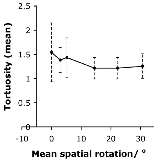
Fig 9. Mean  $\tau$  plotted as a function of the mean spatial rotation,  $\omega$ .
