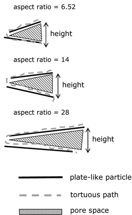
Fig 5. Simplified representation of particle aspect ratio effects on both  $\tau$  and  $\phi$  assuming equal maximum heights between the particles. Both  $\tau$  and  $\phi$  are hypothetical in this schematic.
