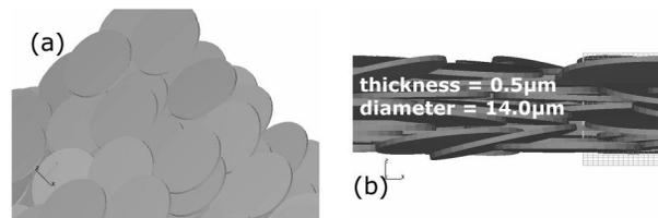
Fig 3. Plate-like packing using aspect ratios of 28 showing (a) a corner perspective and (b) a side view.
