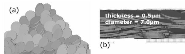
Fig 2. Plate-like packing using aspect ratios of 14 showing (a) a corner perspective and (b) a side view.
