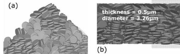
Fig 1. Plate-like packing using aspect ratios of 6.52 showing (a) a corner perspective and (b) a side view.
