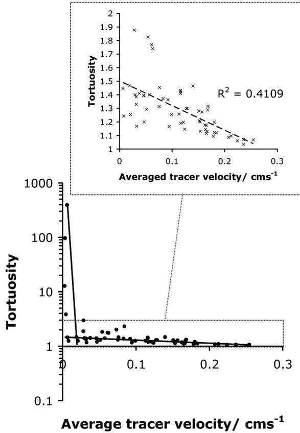
Fig 7. Tracer tortuosity plotted against corresponding mean tracer velocity values.
