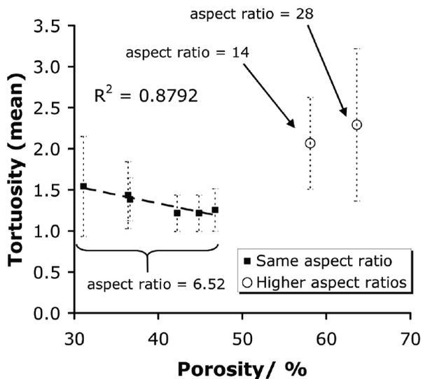
Fig 4.  $\tau$  plotted against  $\phi$  for particle packings with different aspect ratios.
